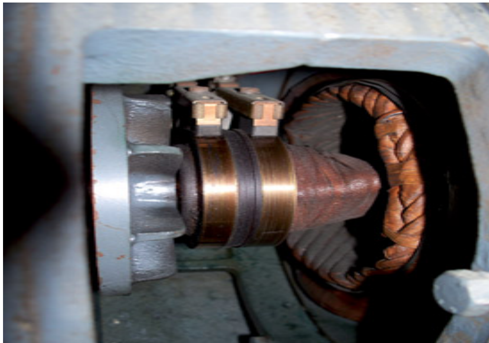
Figure 4-3: Brushes to connect the AVR field voltage to the field rotor
